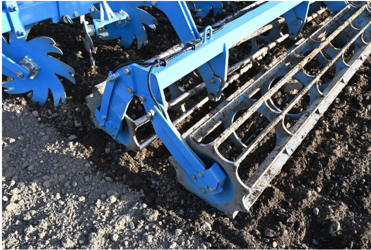
Image 3: LEMKEN iQblue slippage control continuously measures roller slippage.
