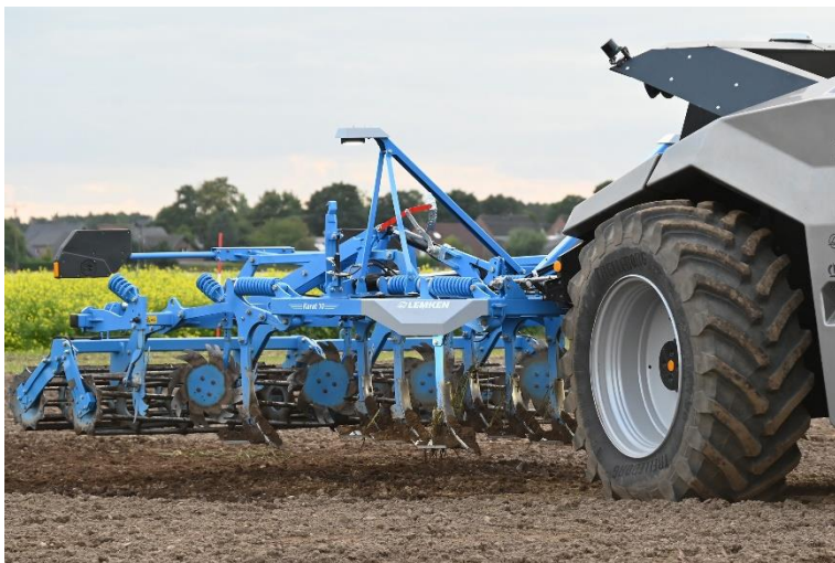
Image 4: LEMKEN iQblue tool management uses a camera with AI-supported image analysis to automatically assess the condition of the cultivator shares at the headland.
