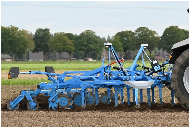
Image 2: LEMKEN iQblue flow control module monitors the flow of material in the tine section in real time.
